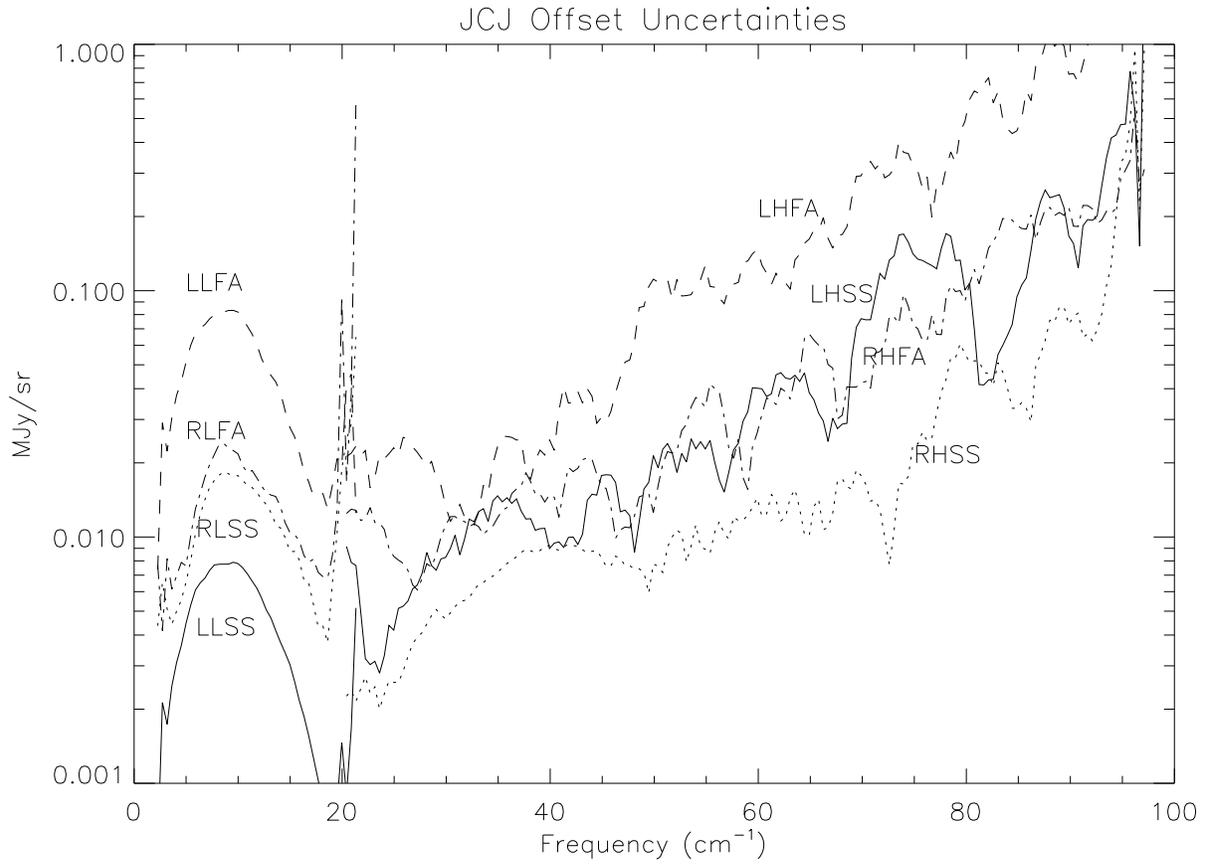
Fig. 7.4.— The *JCJ* offset uncertainties — Derived from the calibration models. The uncertainties reflect the amount and quality of the calibration data.
