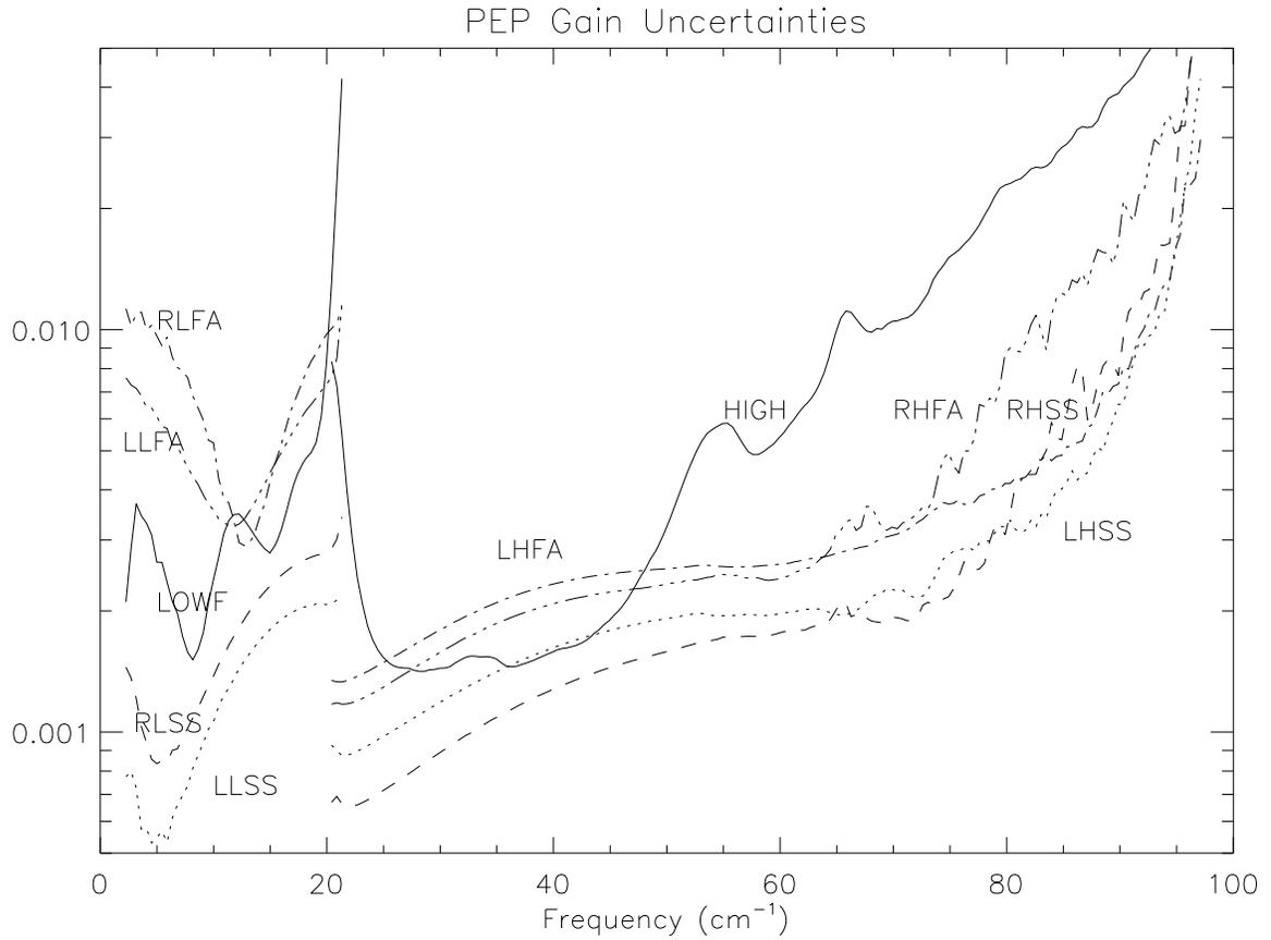
Fig. 7.3.—  $P_gEP_g$  uncertainties — Estimated from the calibration models (LLSS, RLSS, LLFA, and RLFA) and the variation in the calibrated data. Gain uncertainty is dimensionless. The shape of the LOWF estimate is from the “C vector” and so should not be taken too seriously, but the scale is determined from the calibrated data variation.
