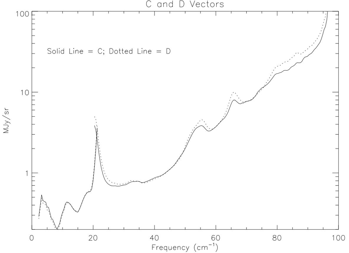
Fig. 7.1.— Relative noise versus frequency —  $C$  and  $D$  vectors for LOWF (2 to 21 $\text{cm}^{-1}$ ) and HIGH (20 to 100  $\text{cm}^{-1}$ ).
