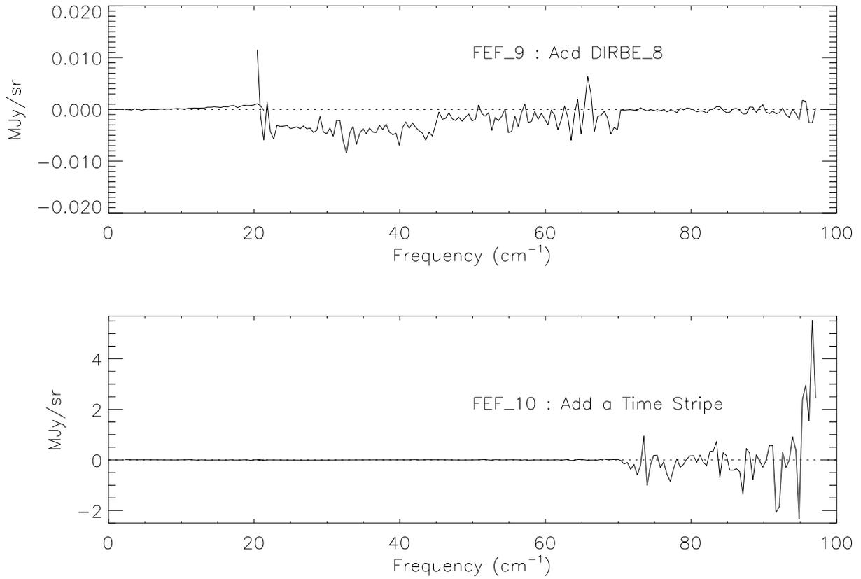
Fig. 7.13.— Additional galactic gradient and time model difference spectra — Average variations in the sky spectra when an additional DIRBE based stripe or an additional time stripe are used. The magnitude of the time stripe difference appears large at high frequencies, but the uncertainties are large there as well. The stripe is not significant by the F test.
