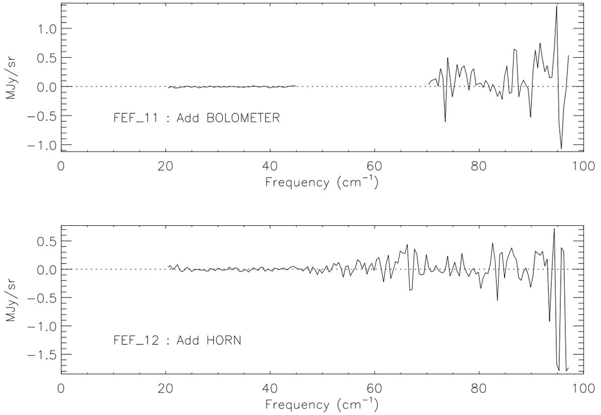
Fig. 7.14.— Additional bolometer and ‘hot horn’ difference spectra — Average variations in the sky spectra when a bolometer stripe, a 4K horn, or 6K horn stripe, for data where such stripes were not used. The additions fail the F test.
