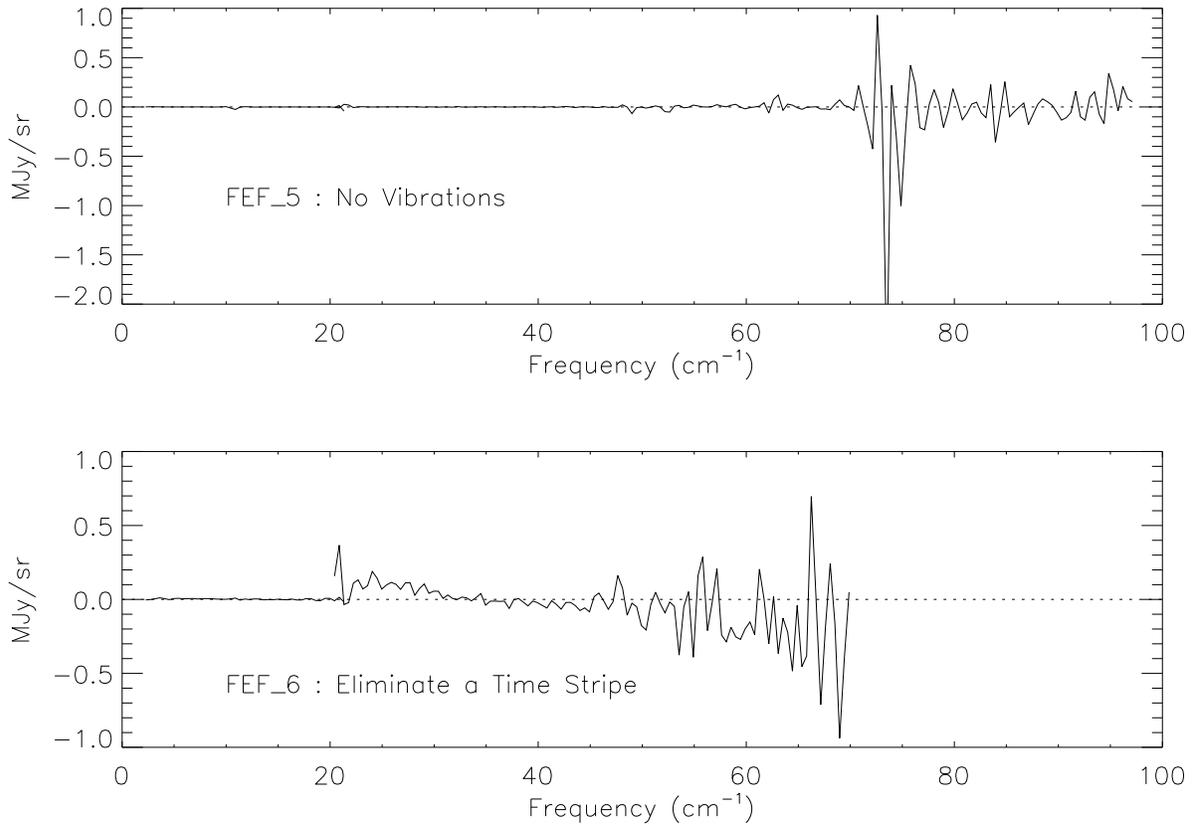
Fig. 7.11.— Vibration and time stripe difference spectra — Average variations in the sky spectra if no vibration stripe was included or if one less time stripe was included. Even though the effect is small in the LOWF, it is still significant.
