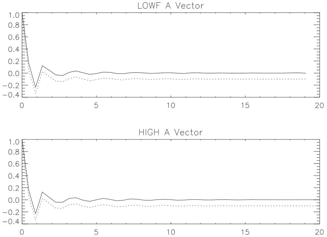
Fig. 7.2.— Frequency-frequency correlations — A vectors for LOWF and HIGH; The solid lines are the “A Vector” estimated from the correlations in the C matrix. The dotted line is the “A Vector” estimated from the apodization, and offset by 0.1 for clarity.
