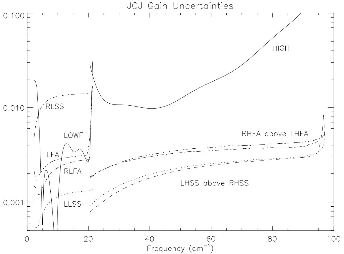
Fig. 7.5.— *JCJ* gain uncertainties — Derived from the calibration models except for LOWF and HIGH which are derived from the calibrated data differences. The dips in the LOWF are probably the result of a chance alignment of the gains.
