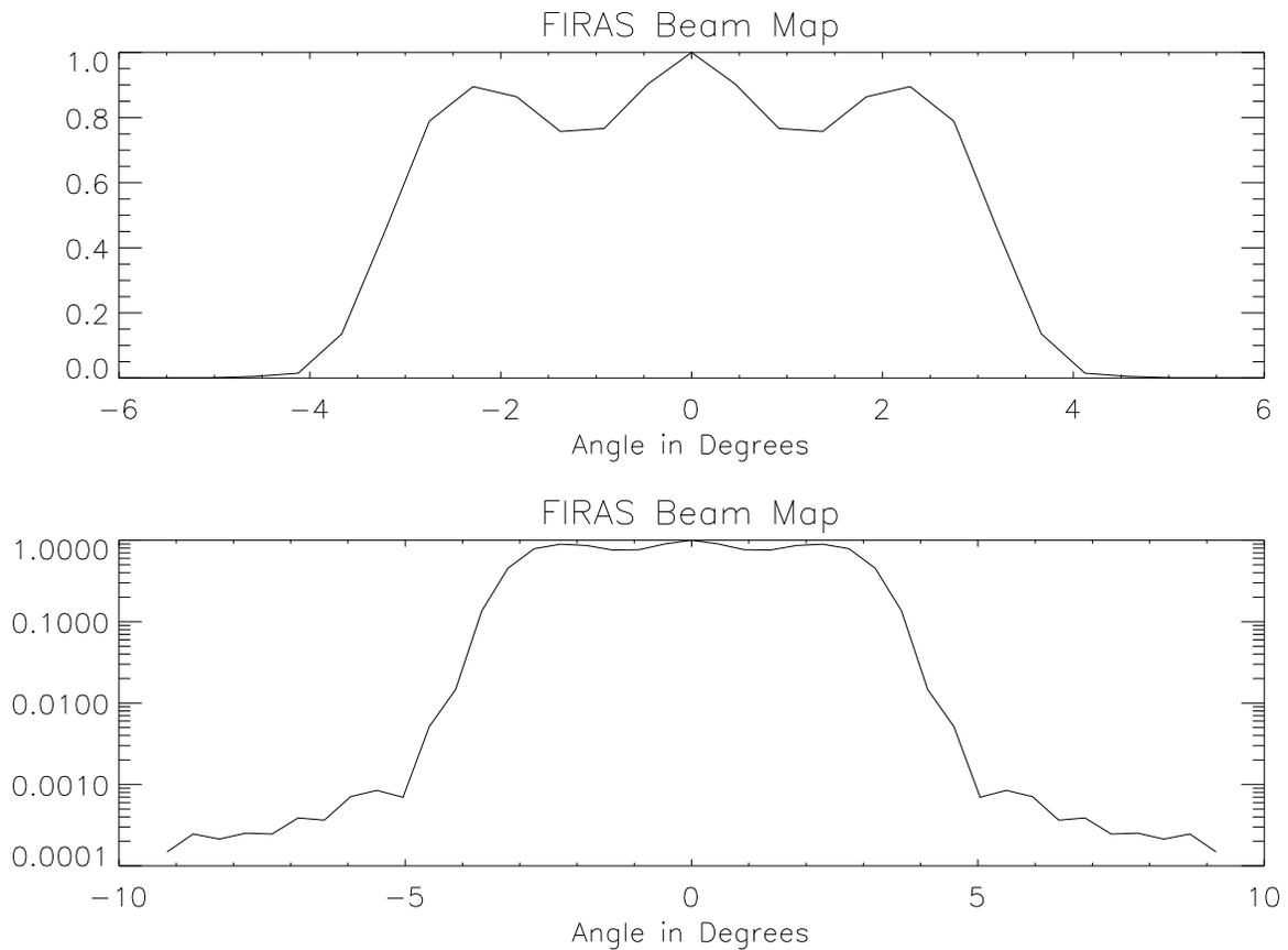
Fig. 7.15.— *FIRAS* beam map — Determined by moon observations. Both linear and logarithmic plots are displayed to show the structure in the beam and the sidelobes.
