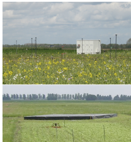
Figure 4: Top: The LBAs of the first LOFAR station in the field. Also visible is the container where the receiving and the local station processing hardware (Figure 5) is located. Below: Six close-packed HBA tiles in the field, with a single HBA antenna element in the foreground.
