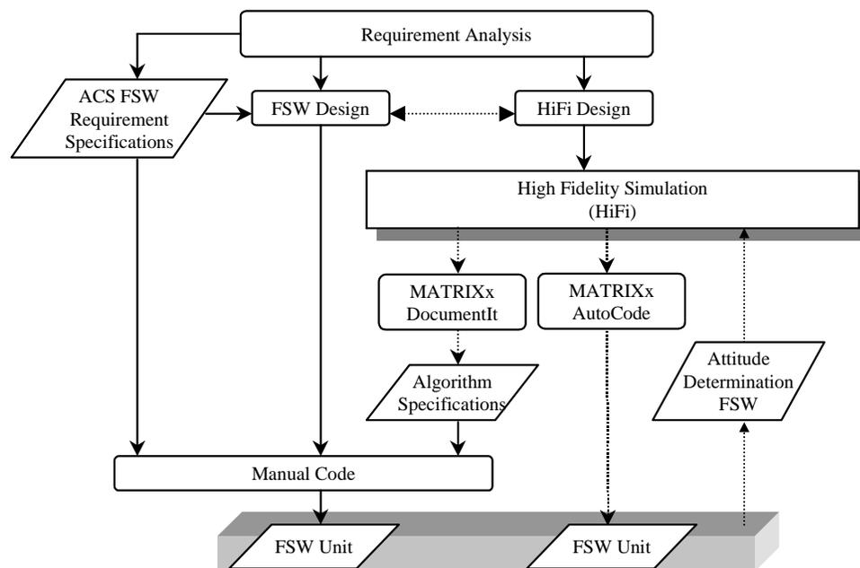
Figure 5: ACS FSW Unit Development Process
